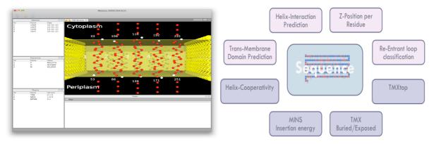
Mebitoo is a platform-independent desktop application written in Java. The software allows to import sequences persistently into an incorporated database engine, namely HSQL. A combined storage concept based on XML-files enables software extensions – plugins – to archive information in customized data structures.
